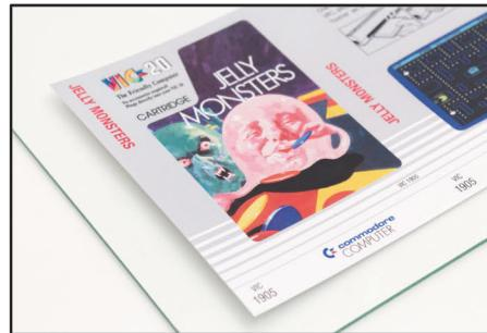
**4** Place the printed sheet on a hard surface (I use a piece of glass from an old scanner). Use the cutter to cut the rectangle of the sleeve. Start from the shorter edges.
